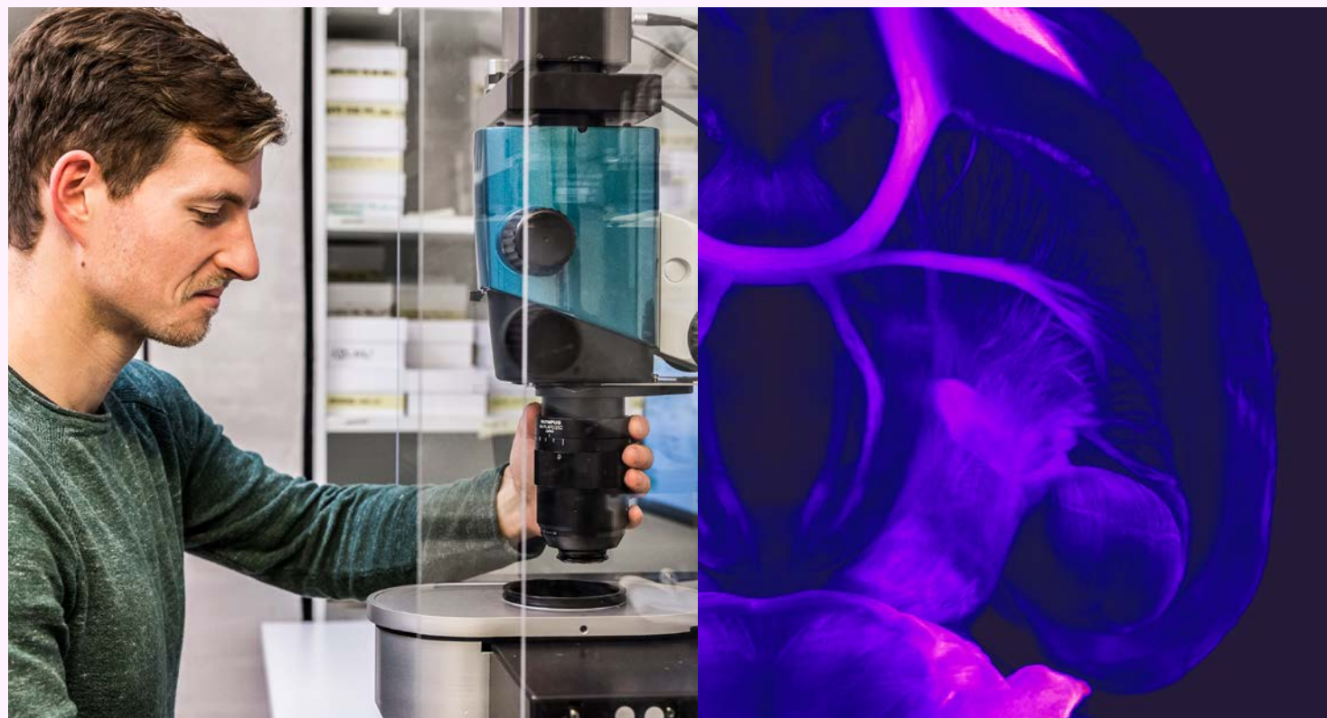
Light-sheet microscope for 3D scanning of large tissue specimens.
